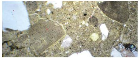
Figure 7.Thin section of lime mortar with sand (3:2 in mixing ratio) from barrel 1, enlarged 50x in polarization microscope. Most of the lime could be beaten and is therefore working as a binder. Lime lumps with hydraulic components exist in a small amount. Photo: Kristin Balksten.
