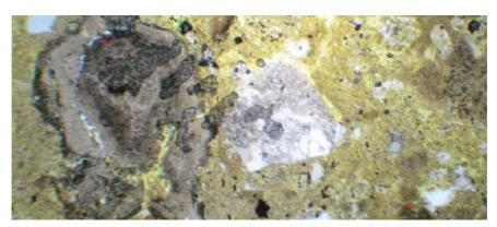
Figure 9.Thin section of lime mortar with sand (3:2 in mixing ratio) from barrel 4, enlarged 50x in polarization microscope. Both sand and hydraulic components act as aggregate in this mortar sample. Photo: Kristin Balksten.
