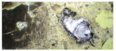
Figure 8. Thin section of unbeaten lime from barrel 4, enlarged 50x in polarization microscope. The lime paste is inhomogenous with distinct lime lumps of hydraulic components. The sample looks as if it contains some aggregate rather then pure lime, which is the hydraulic components that has hardened over two hundred years. Photo: Kristin Balksten.
