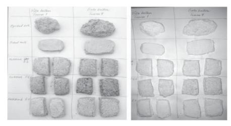
Figure 5.The experimental samples when they are fresh (to the left) and after two weeks (to the right), when they have been dried white. The samples that seamed very lean as fresh appeared more lime rich after hardening. Photo: Kristin Balksten.
